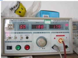
2.Earth Test:  $10A < 50m\Omega$ , The result is ok
